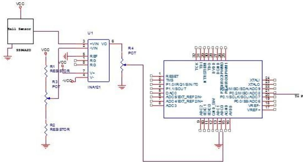
Figure 3: Circuit diagram of Magnetic field measurement
