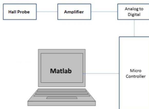
Figure2: Magnetic Field Measurement System Block Diagram
